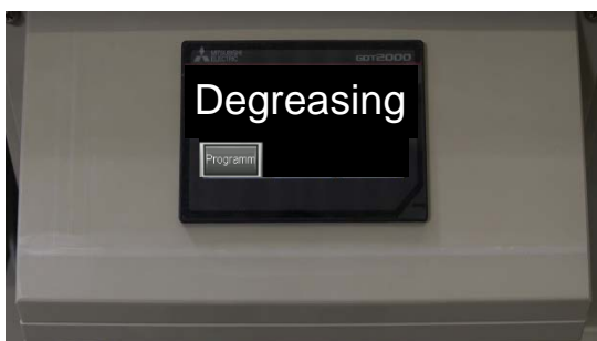
Control panel for process control (Example: degreasing)
